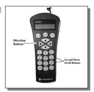
Input the necessary date and time information as instructed by the hand control. Press ENTER after each entry. The NexStar will also ask for time zone and location information. Use the UP and Down scroll buttons to select from the various options, pressing ENTER after each selection. (See *Hand Control* section for detailed alignment procedures).
